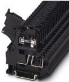
Fuse terminal block for assembly on NS 35, for 5 x 20 cartridge fuse inserts
